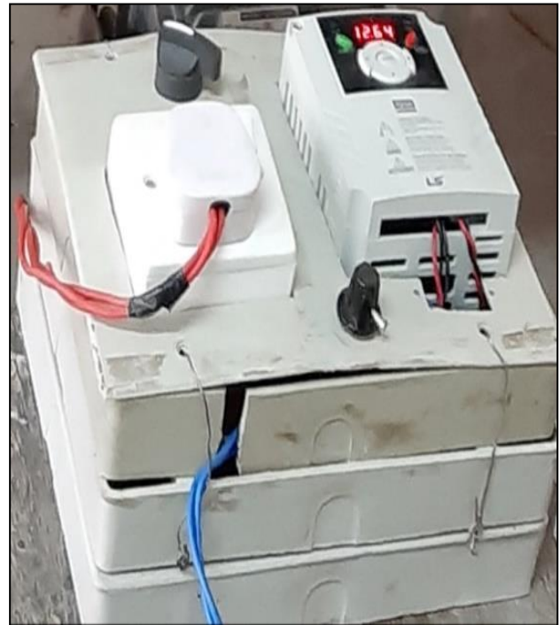
Figure 5: Image of a) an inverter b) circuit of inverter with seat suspension system
